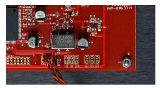
For jumper settings, see below. Make sure that you have the latest firmware uploaded in your Hydra Z. Present settings are for firmware 1.06. If you have no sound or distorted sound over the I2S output, alter J22 or J24..26 setting.
